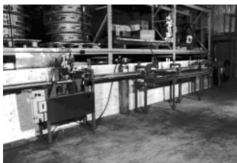
Sunstrip™ inflation machine Operation: uncoil, inflate and cut SS146/12 fin
